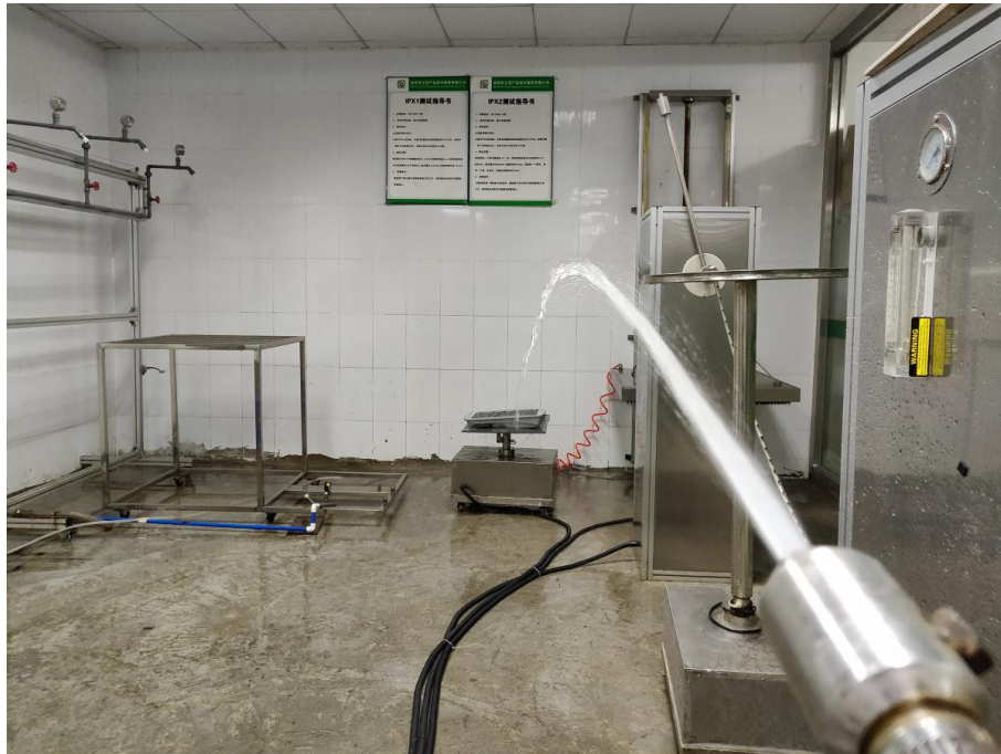
Photo 3: IPX5 test of model TLSTC08XYZZ
