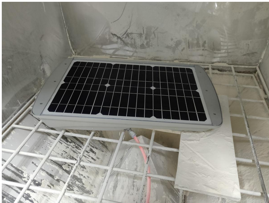
Photo 2: IP6X test of model TLSTC08XYZZ
